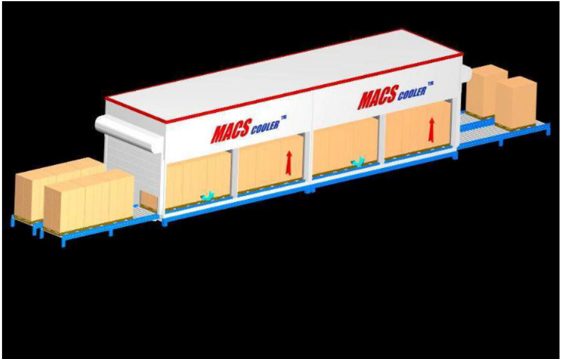
Section view of MACS Cooler with Product loaded on Infeeds, Zones 1-4, and Outfeeds. Rendered in AutoCAD 3D.
